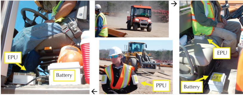
Figure 5. Alert devices on personnel and equipment during field experiments
