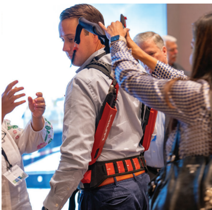
Attendees try on the new Hilti Exoskeleton designed to help relieve shoulder and neck fatigue when working above shoulder level.
